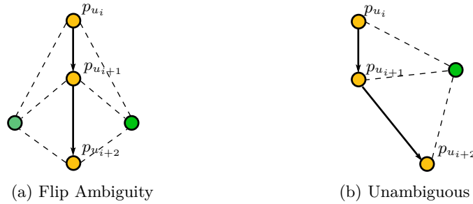
Fig. 5: Moving robot (yellow/light gray) localizing a stationary robot (green/dark gray) using distance measurements (dashed lines) and odometry (solid arrows).
