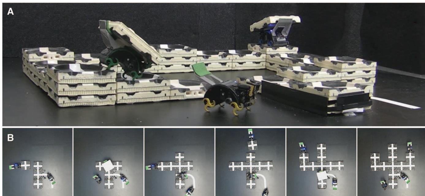
Fig. 4. Hardware demonstration. Independent autonomous robots with purely onboard sensing collectively work on prespecified structures. (A) A castle-like structure (movie S3). (B) A sequence of overhead snapshots building a branching structure (movie S4).
