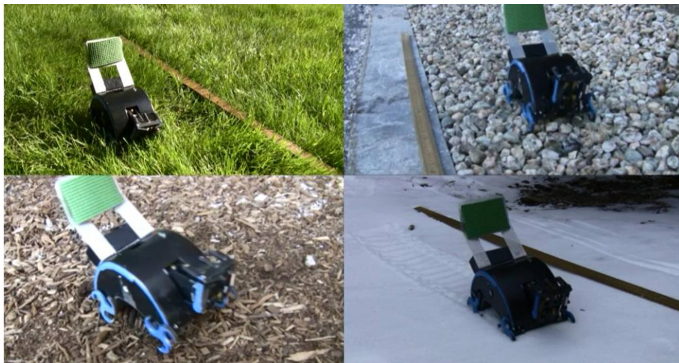
Figure 4.8.a. Exploiting whigs, the robot is able to traverse various surfaces with simple control.
