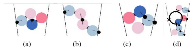
Fig. 10: Bridge dissolution failures: (a) A bridge robot grabbed from below (b) Two bridge robots grabbing each other (c) Walking (top) robot stuck in the terrain (d) Trapped walking robot which moves in circles
