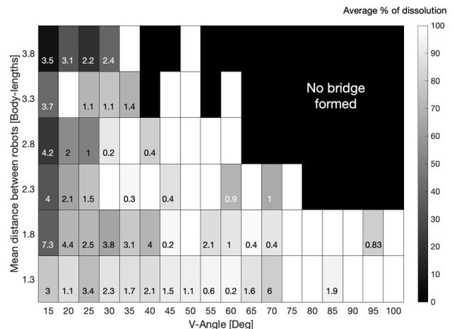
Fig. 9: Bridge dissolution across different terrain and traffic
