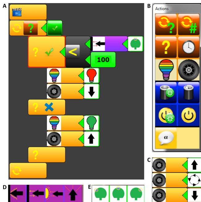
Fig. 3. Graphical programming language, based on Miniblog (miniblog.org). (A) A simple example program. The robot will turn its LED red and back up if it detects an obstacle too close to its center distance sensor; otherwise it will turn its LED green and move forward. (B) The action pane, giving categories of blocks that can be used to start a new statement: while loops, for loops, conditionals, delays, LED-color commands, motor commands, variable initialization and variable assignment (both floating-point and Boolean), comments. (C) A block starting a statement provides a context-specific selection of blocks to continue the statement: e.g., a motor block can be followed by a block specifying forward, left, or backward movement. (D–E) Different blocks specify the type of sensor (D: bump, distance, ambient light, line) and its location (E: left, center, right).
