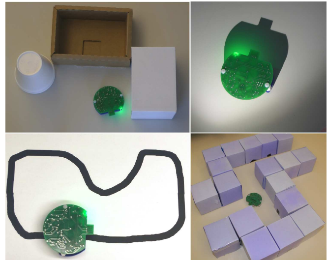
Fig. 1. Examples of behaviors the AERobot can be programmed to perform. Clockwise from bottom left: line-following, wall-following, phototaxis, maze-solving.
