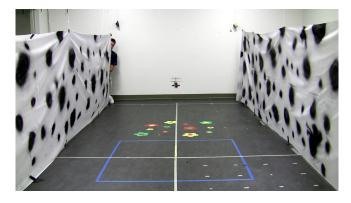
Fig. 5. A photograph of the corridor-like environment within the Vicon arena during an experiment. The dimensions of the corridor were approximately 5.0 m  $\times$  2.6 m  $\times$  1.5 m ( $L \times W \times H$ ).
