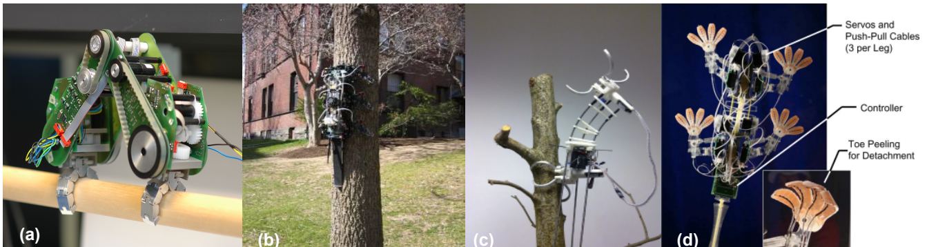
Figure 1.7: different ways of gripping and attaching : (a) bipedal robot with 2 grippers [35], (b) RiSe robot [39], (c) Treebot [34], (e) GeckoBot [40]
