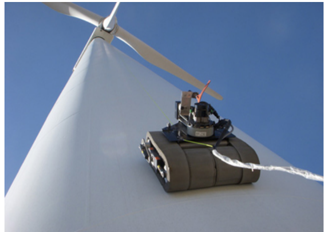
Figure 1.4: ICM wind turbine inspection robot using vacuum to climb on brick, metal, or concrete [21]
