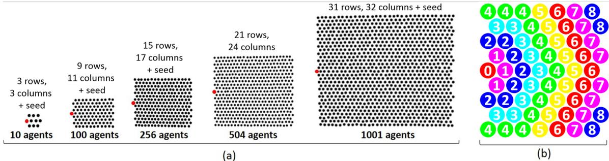
Figure 2: (a) Arrangement of agents and seed locations in experiments with several collective sizes; (b) Gradient values and display color scheme for an ideal (i.e. error-free) scenario. The red agent with a gradient value of 0 is the seed.
